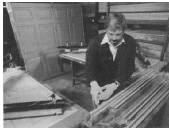
FIGURE 36.14 Mild steel stiffeners are bonded to up and over garage door. Result: rigidity; unblemished exterior surfaces.
