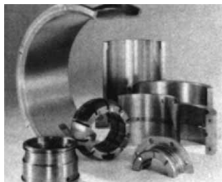
FIGURE 35.8 Thick walled bearings are produced as bushes, half bearings and thrust washers in copper and aluminium base alloys, also tin and lead base whitemetal.
