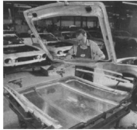
FIGURE 36.13 A structural adhesive used to bond a stiffener to an aluminum car bonnet. To line up the two parts a purpose made fixture is designed.
